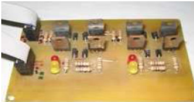
Fig. 8. Print circuit board of motor driver circuit.
